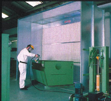
Typical three tier dry filter spraybooth
